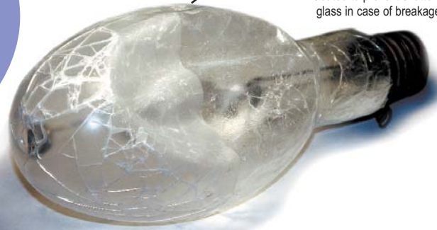
Coated to prevent shattered glass in case of breakage.
