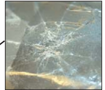
Coated to prevent shattered glass in case of breakage.
